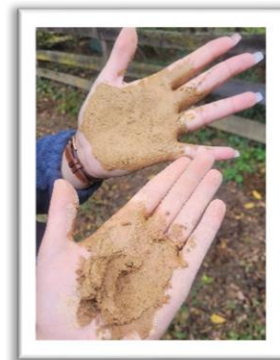
Texturing Soil Out to Help Pinpoint Where Water Issues Were Originating
