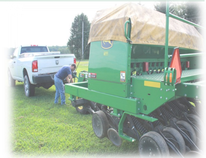
Ag Resource Specialist Ben Smith hooking up one of the John Deere No-till Drills.
