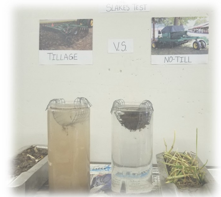
The Slakes Test in action, exemplifying soil stability.
